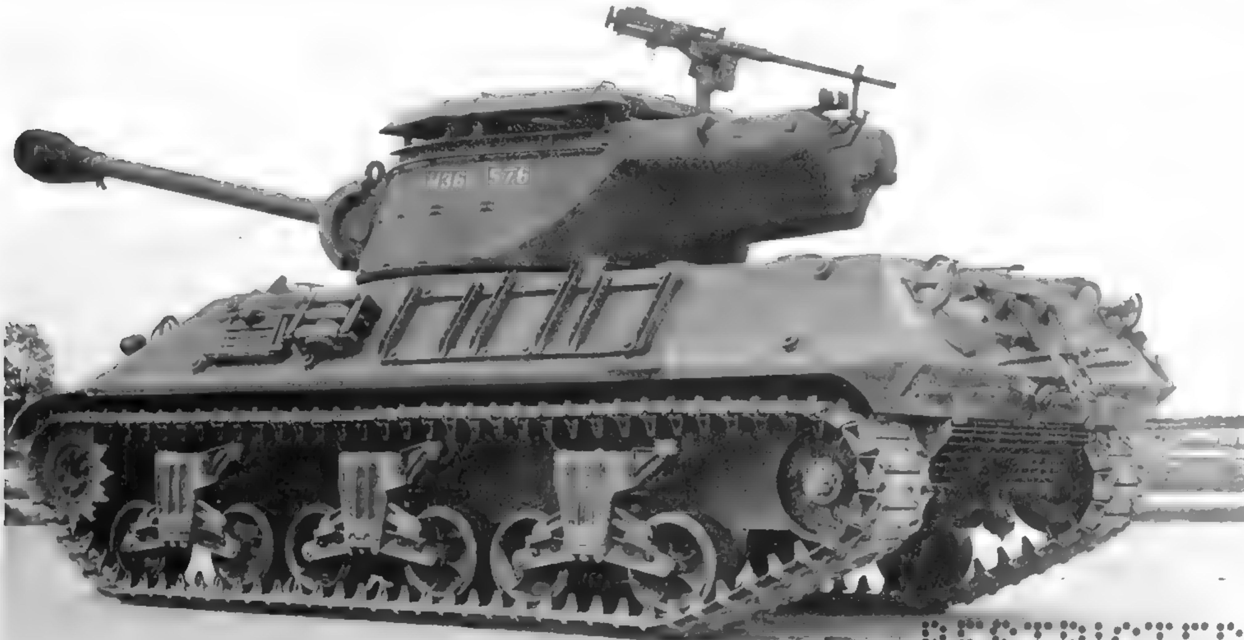
The M36 was basically an upgunned M10 Tank Destroyer. The new gun was a 90mm weapon, and its gun tube seemed disproportionately large for the chassis. (Photo courtesy of the Patton Museum)
